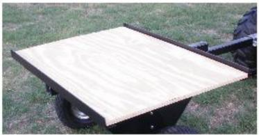
Step 12 Trailer must be decked with plywood and feeder bolted through plywood and trailer on corners. (Plywood NOT INCLUDED)
