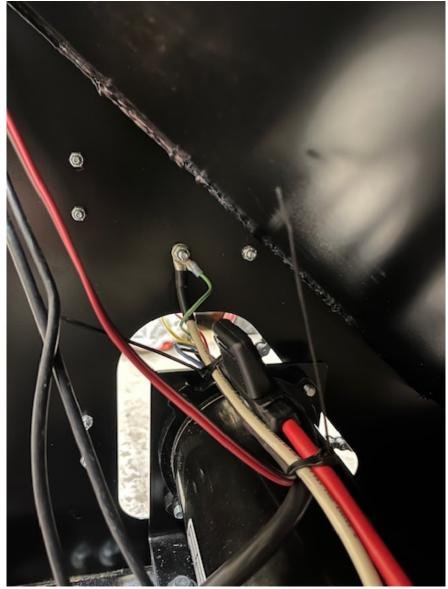
You can use the same bolt that your motor ground is attached to for the green gound wire
